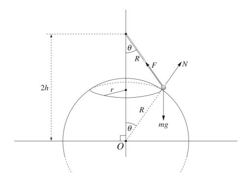
Three forces act on the bead: the tension force F of the string, the normal reaction force N to the surface of the sphere, and the gravitational force mg.
